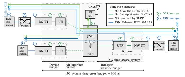
Fig. 1. Time synchronization in 5G-TSN network where 5GS operates as a time-aware system. Time synchronization for downlink GM (dark blue), uplink GM (light blue) and 5G GM (green) are provided. The GMs are represented with small colored dots.
