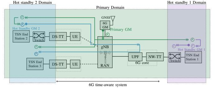
Fig. 3. 6G GM as primary GM and one hot standby GM on device-side TSN end station and another hot standby GM on network-side TSN end station.
