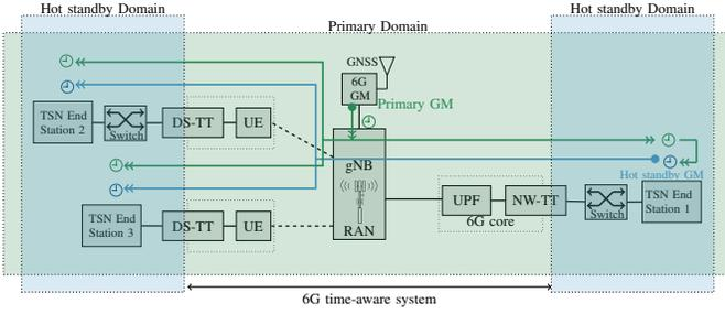
Fig. 2. 6G GM as primary GM and network-side TSN end station as hot standby GM.
