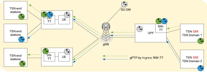
Uplink direction: Grandmaster GM is behind a Device (Rel-17)
