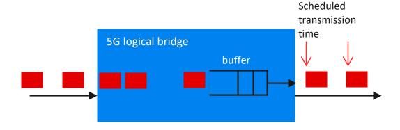
□3GPP does not specify how the Hold and Forward buffers should be implemented
